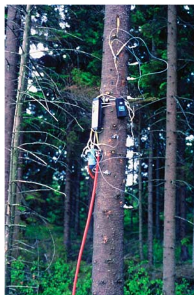
Fig. 18 Spruce tree ( Picea abies ) with small glass tubes fitted to bark beetle entrance holes and with a minipump (centre right) and a larger pump (at the bottom end of the red tubing) to collect emitted volatiles through adsorption.
